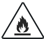
Caution: Risk of fire
